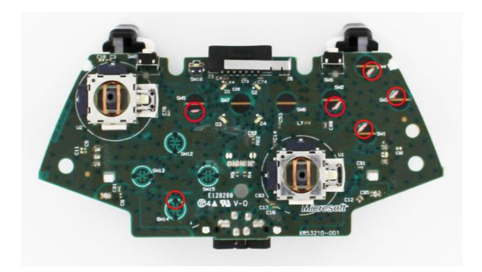
The CG1 is the most common board currently found. It looks very similar to the CG2 board, only with the black Microsoft chip on the back of the controller being at a 45 degree angle, instead of square on. The install for that is identical to the CG2 board, so we only show the images for the CG2.
