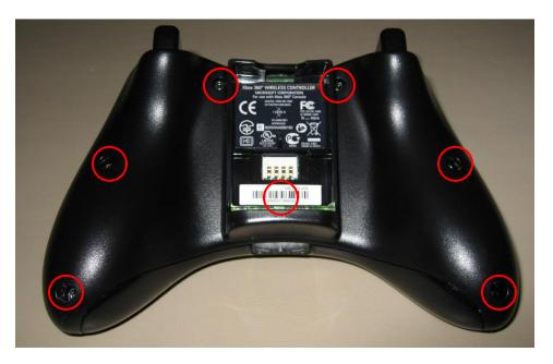
*Note: One of the screws is located beneath the barcode sticker in the battery compartment. This sticker can be removed by scraping at the edge with a razor blade or small screwdriver.*
