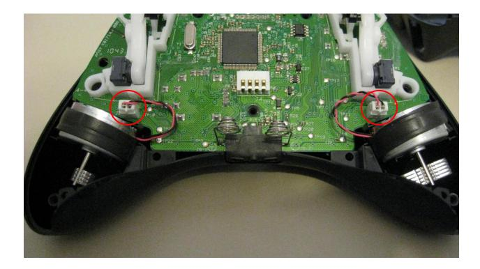
Step 4: Remove circuit board from controller case by pushing the joysticks through the top half of the case.
