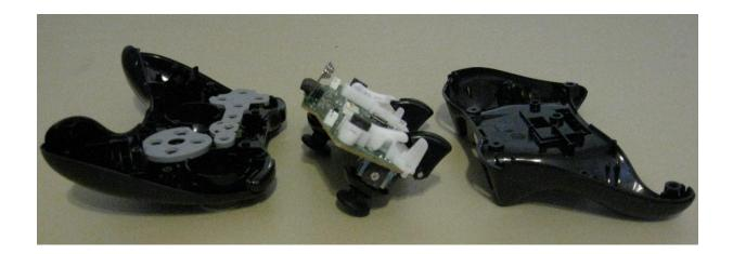
Step 5: Remove joystick covers to keep from accidentally melting them with the soldering iron during the install. Pull joystick covers straight up and away from board to slide off.
