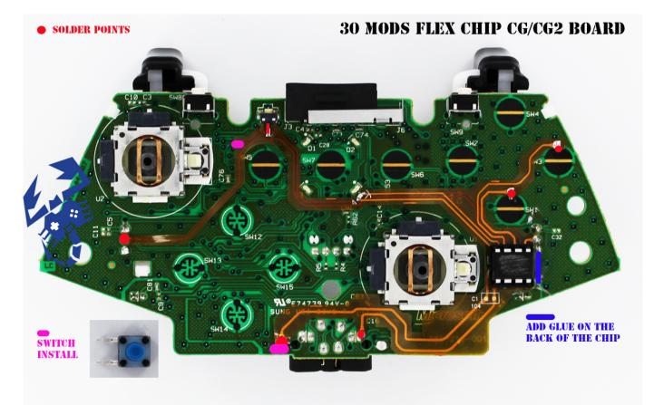
The next steps walk you through wiring the mod. Here's a schematic.
